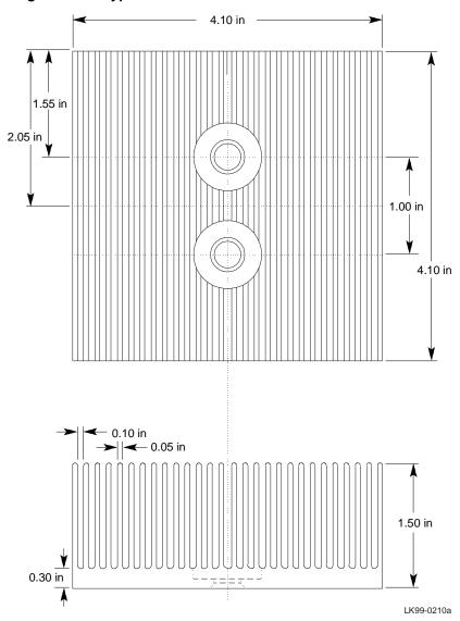
Figure 10–2 shows the heat sink type 2, along with its approximate dimensions.
