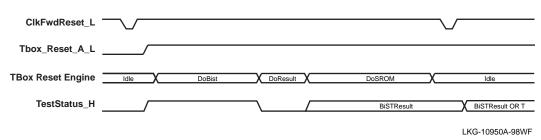
Figure 11-1 TestStat H Pin Timing During Power-Up Built-In Self-Test (BiST)
