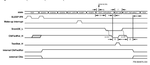
Figure 7–3 Sleep Mode Sequence of Operation
