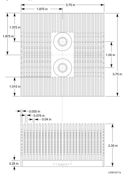
Figure 10–3 shows heat sink type 3, along with its approximate dimensions.
