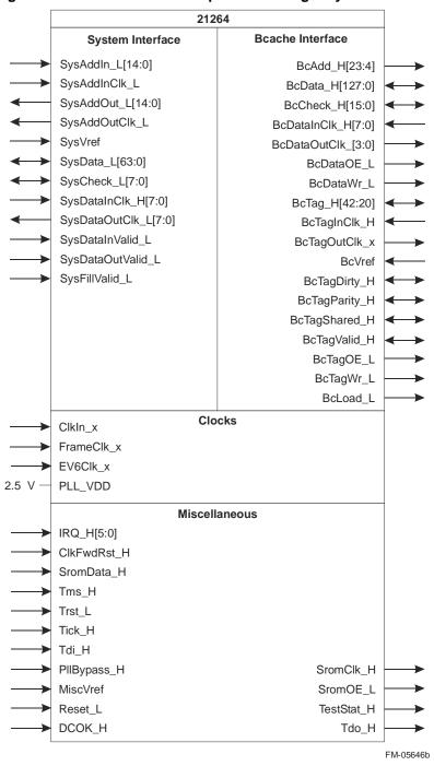
Figure 3-1 21264/EV68A Microprocessor Logic Symbol
