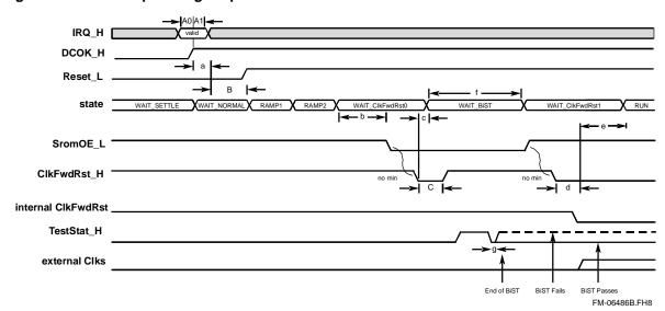
Figure 7–1 Power-Up Timing Sequence
