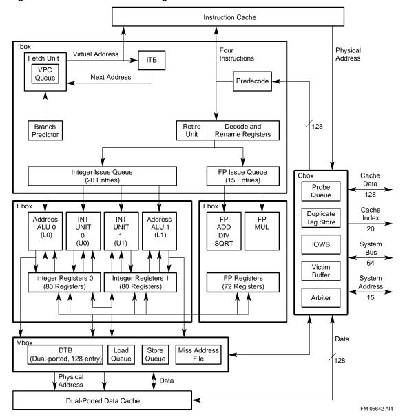
Figure 2-1 21264/EV68A Block Diagram
