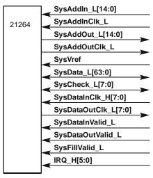
Figure 4–4 System Interface Signals
