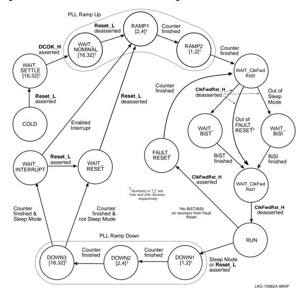
Figure 7–5 21264/EV68A Reset State Machine State Diagram
