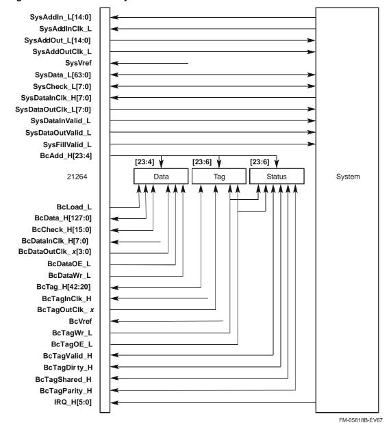
Figure 4-1 21264/EV68A System and Bcache Interfaces
