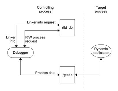
FIGURE 6-1 rtld-debugger Information Flow
