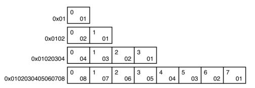
FIGURE 7–2 Data Encoding ELFDATA2LSB
