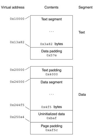
FIGURE 7–10 32-bit SPARC: Process Image Segments
