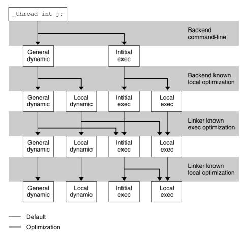
FIGURE 8-2 Thread-Local Storage Access Models and Transitions
