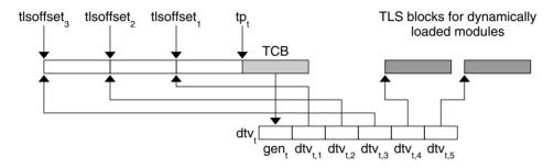
FIGURE 8-1 Runtime Storage Layout of Thread-Local Storage
