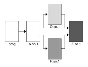
FIGURE 3-3 Multiple dlopen() Requests With A Common Dependency
