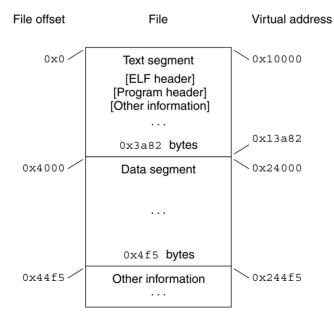
FIGURE 7-8 SPARC: Executable File (64K alignment)
